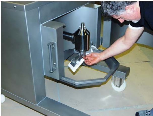
Fig. 13: Installing the scraper unit
