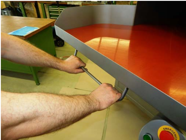
Fig. 24: Lifting the chute
