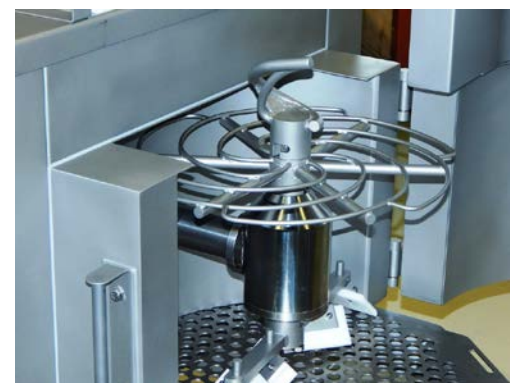
Fig. 18: Pre-separator hook mounted
