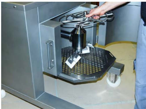
Fig. 15: Mounting the spiral separator Spiral separator mounted
