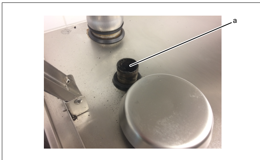
Image: Combisteamer with the smoker box removed
