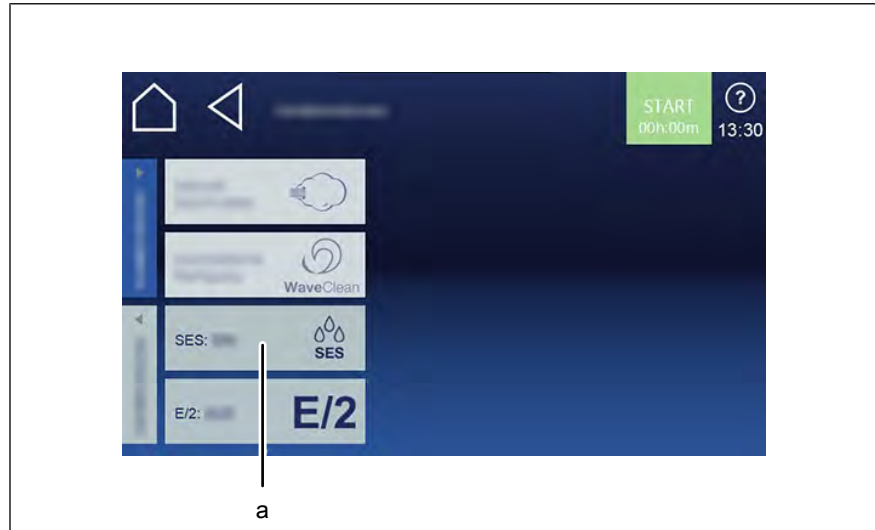
Image: Steam Exhaust System (SES) selection window
