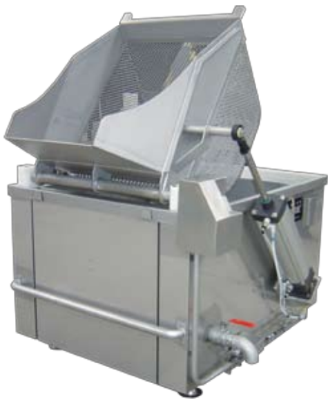
Cooker type 500, steam heat exchanger.
