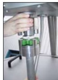
Inclined, removable scraper arm and satellite mixer.
