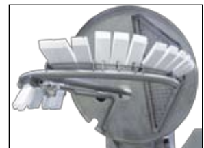
Inclined, removable scraper arm and satellite mixer.
