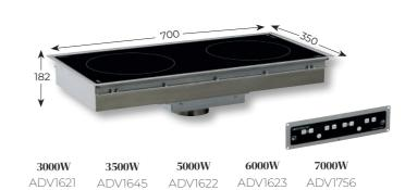
Product cut-out dimensions 333 x 692 mm Control panel cut-out dimensions 60 x 302 mm
